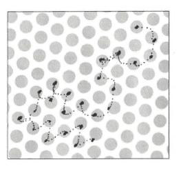
This graphic shows the trajectory of the STM tip as it tracks a water molecule in its random hopping from one nearest neighbor lattice point to another across the crystal of a palladium surface. The image was produced at 52.4 Kelvins.
